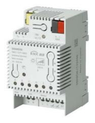
The universal dimmer main module N 527/31 is an installation device for DIN-rail mounting, with N-system dimensions. It is designed for lighting control, i.e. for switching and dimming resistive, inductive or capacitive loads from 20 to 500 VA at 230V AC, 50-60 Hz. The bus is connected via a bus terminal and the power supply for the electronics is provided by an integrated 230V AC power supply unit.
