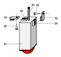
Figure 2: Wall and ceiling mountings
