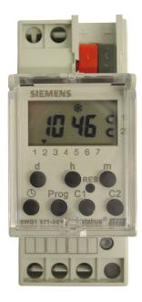
The 2-channel time switch REG 371 (weekly scheduler) with integrated bus coupling unit is a DIN rail mounted device for mounting in distribution boards. The connection to EIB is made via a bus connector.
