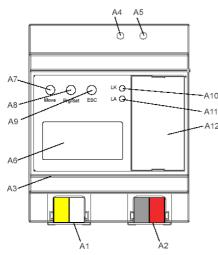
Figure 1: Location of the display and operator elements
