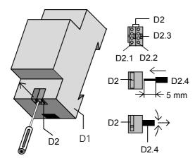
Figure 3: Connecting and disconnecting bus wires
