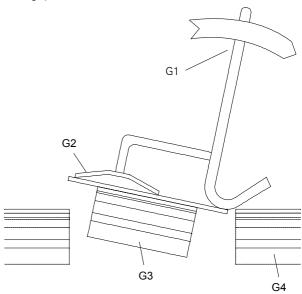
Figure 8: Direction of leverage for dismounting
