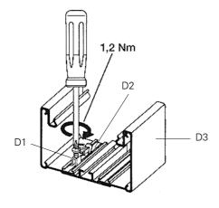
Figure 4: Tightening the earthing clamps
