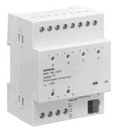
The zone terminal N 266 is a DIN rail mounted device with N-system dimensions and a width of 4 module units. It is used for the monitored connection of passive detectors to the *instabus EIB* and/or to connect floating contacts in applications with increased security requirements (e.g. monitoring of the sensor line).
