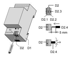
Figure 3: Connecting and disconnecting wires
