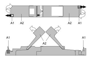
Figure 2: Opening and closing the cover lids
