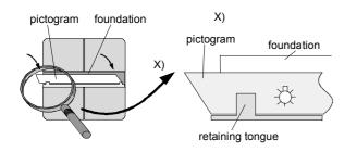
Diagram 7: inserting the pictograms
