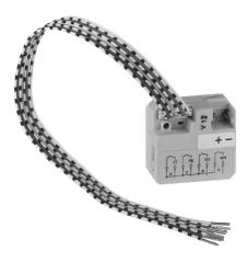
The push button interface UP 220/02 is a binary input device for use with box mounts (Ø 60 mm, depth: 60 mm). 4 inputs are available for volt free switching/ keying contacts. The required scanning voltage is provided by the push button interface (requires no additional power supply).
