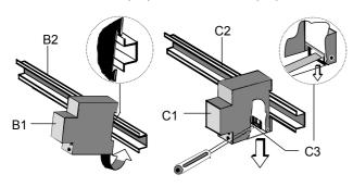
Figure 2: Mounting and dismounting a DIN-rail device
