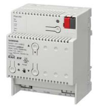
The KNX / DALI gateway N 141/02 is a 4 MU wide, DINrail mounted KNX device with one DALI interface to which up to 64 DALI actuators (e.g. DALI ballasts) can be connected to. It is not allowed to connect DALI sensors to the DALI interface of the N 141/02.
