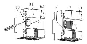
Figure 4: Covering the contact system
