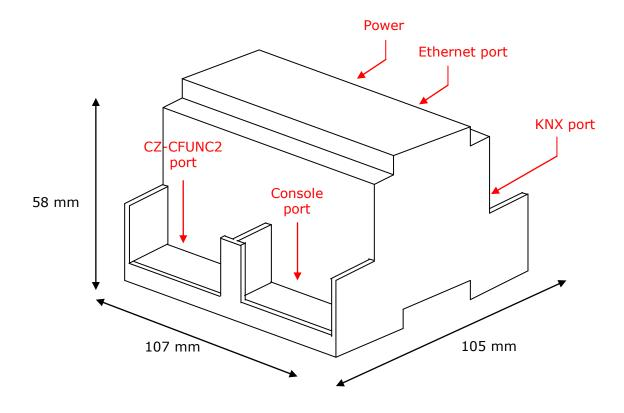
Free space recommended in the install location of the device, with spacing enough for external connections.
