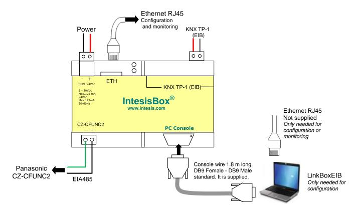
Standard cable DB9male-DB9female 1,8 meters long is supplied with the device for connection to a PC COM port for configuring and monitoring the device. The configuration software, compatible with Windows® operating systems, is also supplied.
