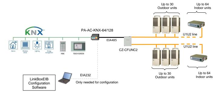
IntesisBox is a KNX device, capable of monitoring and controlling Panasonic ECOi and PACi indoor units connected to a Panasonic CZ-CFUNC2 communication adaptor<sup>1</sup>. Up to 64 indoor units and 30 outdoor units can be integrated within a single channel. If you use both channels, up to 128 indoor units can be integrated.
