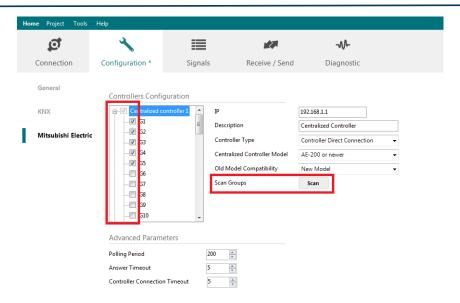
Figure 4.5 Selection of active groups in Centralized Controller
