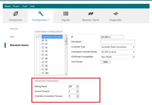
Figure 4.9 Advanced Parameters for communication with Centralized Controllers
