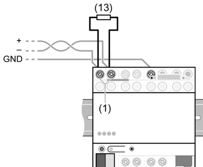
Fig. 4.2-2: Terminating resistance
