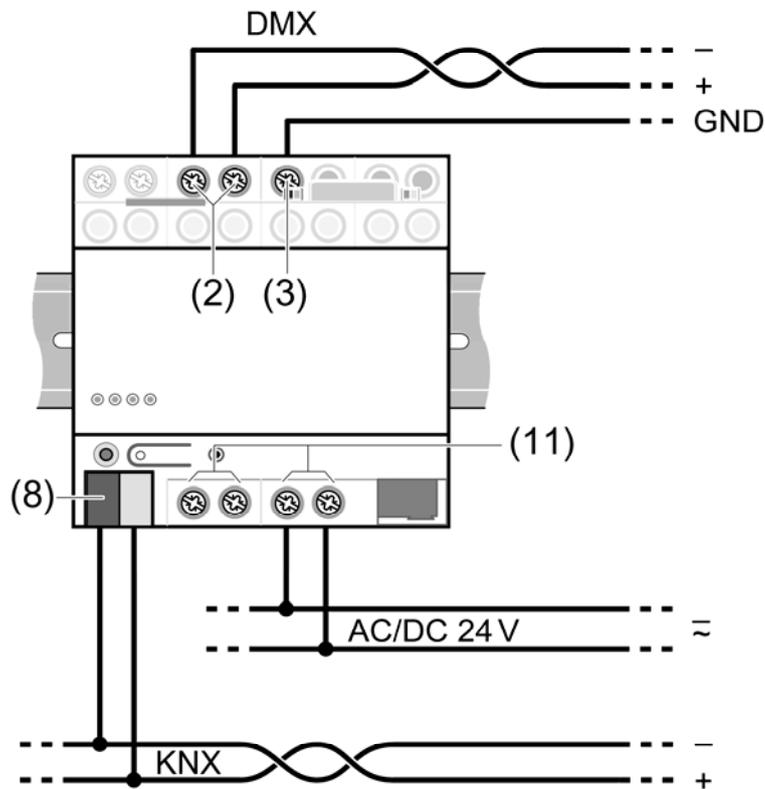
Fig. 4.2-3: Connection – Operation mode Master
