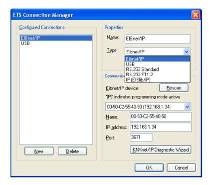
To be able to access KNX/EIB, the KNX IP Interface 730 requires an additional physical address. This second physical address is only used for bus access and must be set up separately:
