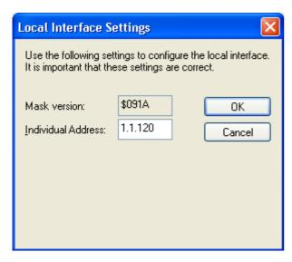
Enter a physical address of your choice. A dummy device may have to be added to the ETS project to reserve this address.
