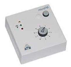
There are **3 Programmable LED's**, a **10 Step-Switch** and one Pushbutton. MicroFM will also be delivered optionally with an integrated DCF77 - Time - Signal Receiver.
