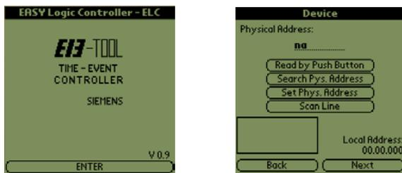
The program connects to the bus and support the search for N350 and N341 modules with different methods: search for devices with pressed programming button, scan a line, or direct entry of the physical address of a module.
