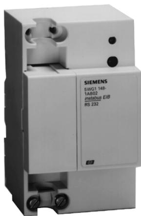
The N 148 interface with its built-in Sub D 9-pin plug-and-socket device, enables a personal computer (AT compatible PC) to be connected for addressing, parameterising, visualising, logging and diagnosis of bus devices.
