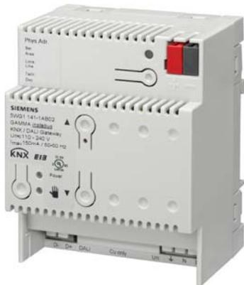
The KNX / DALI gateway N 141/02 is a 4 MU wide, DIN-rail mounted KNX device with one DALI interface to which up to 64 DALI actuators (e.g. DALI ballasts) can be connected to. It is not allowed to connect DALI sensors to the DALI interface of the N 141/02.
