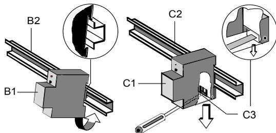
Figure 2: Installing / dismantling the DIN rail mounted device
