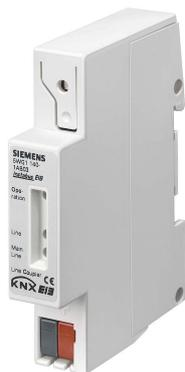
The line-/ backbone coupler N 140/03 provides a data connection between two separate EIB bus lines and also isolates the bus lines from each other in order to enable the independent local operation of a bus line.
