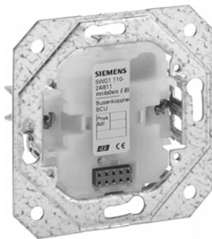
The bus coupling unit (BCU) UP 110/11 enables application units (AUs) to be connected to the bus line via the physical external interface (PEI). The telegrams received via the bus line are processed by the BCU and passed on to the application unit. In the opposite direction, signals coming from the application unit are converted into telegrams and transmitted.
