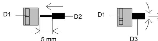
Figure 4: Connecting/disconnecting a bus cable
