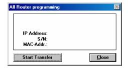
By pressing of the "Start transfer" button the data communication starts. The data will be sent using your local network. For this reason all EIB routers must have a valid IP address, which corresponds to the configured, and need to be connected to the network and supply voltage. If errors arise, you should examine the EIB routers and afterwards repeat the programming process.
