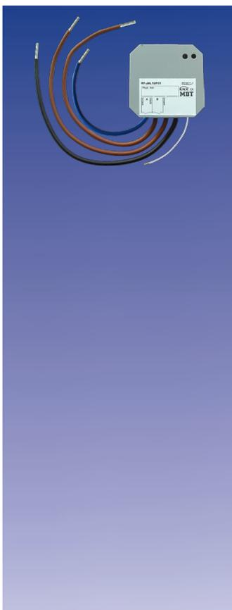
**KNX RF Shutter Actuator 1-fold, flush mounted, 6A, 230VAC**
