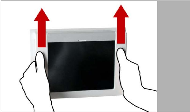
Push the upper section of the housing (frame with display) up a little and lift it off.
