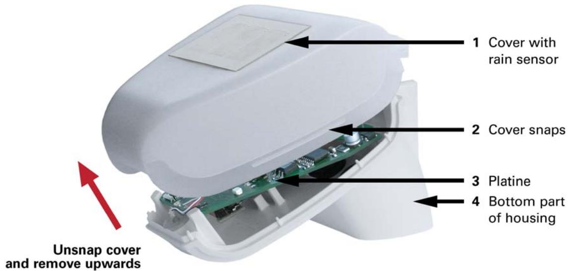
The weather station lid with the rain sensor latches into place on the lower edge to the right and left (see diagram). Remove the lid from the weather station. Proceed carefully to avoid tearing off the cable connection between the circuit board in the lower section and the rain sensor in the lid (cable with plug).
