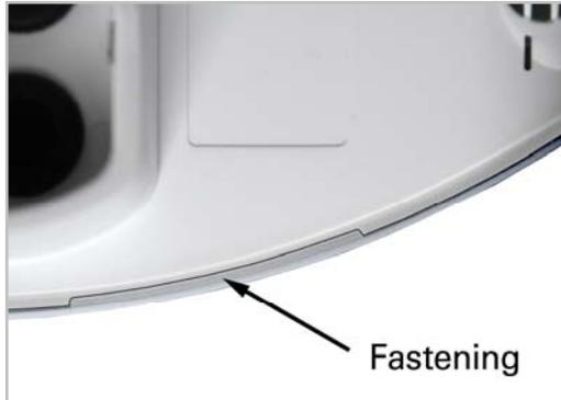
Check that the lid and lower section have properly latched into place! The diagram shows the closed weather station from below.
