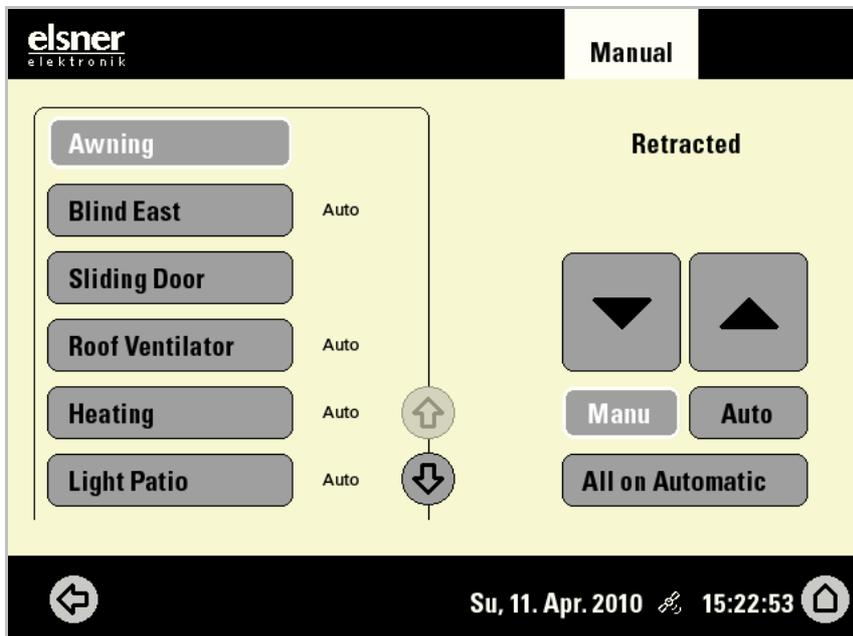
Here you can operate all connected drives and devices directly: Use the buttons to select the name of the drive or device you want to operate. You can change the order of the list in the System menu.
