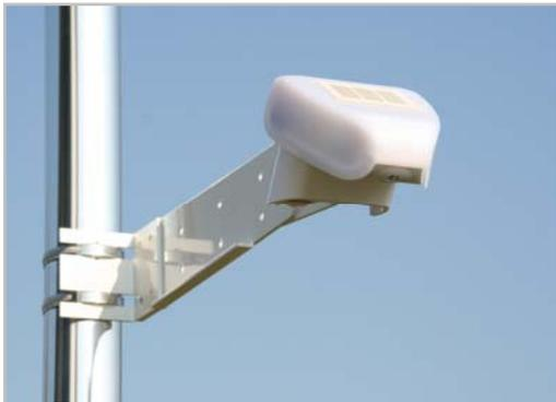
Example 2: Fitting to a pole with worm drive hose clips
