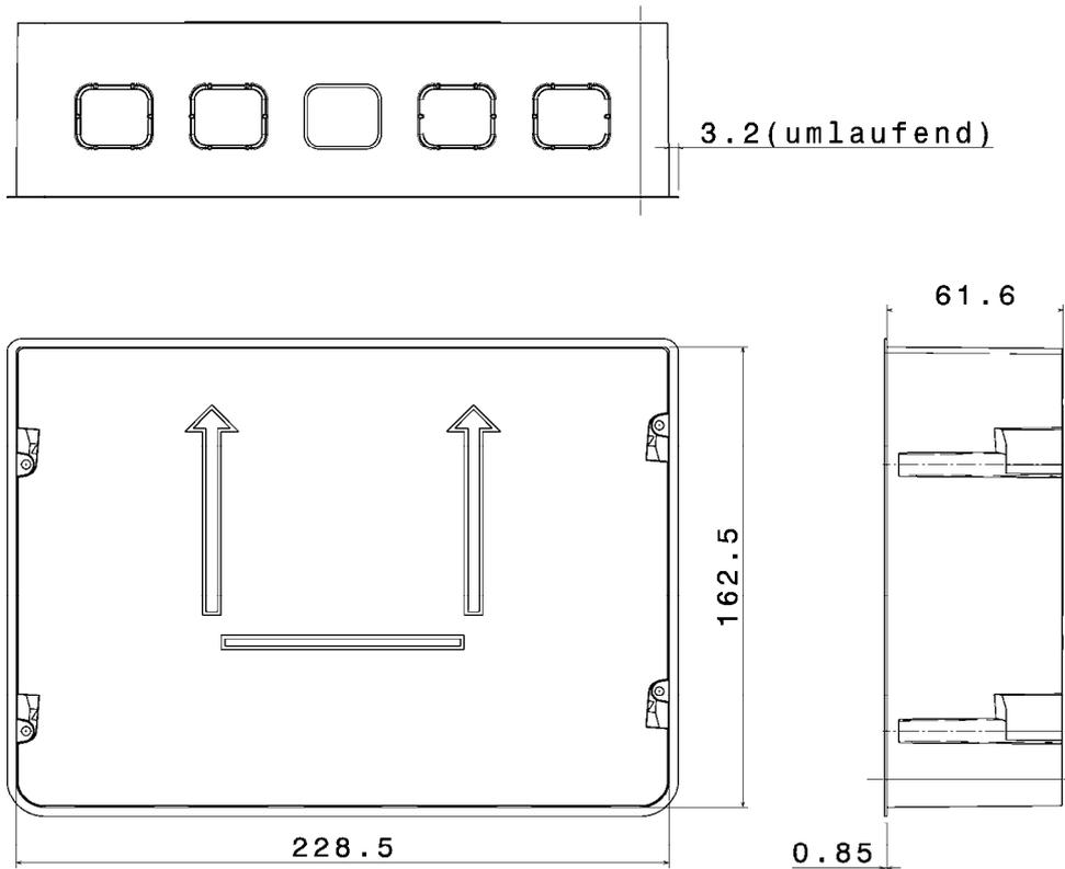
Cut-out dimensions for flush-mounted casing:
