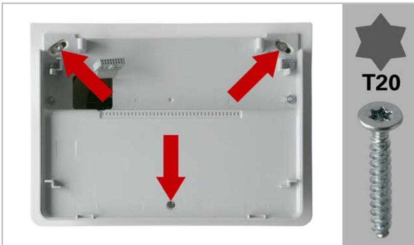
The lower section of the housing together with the wall-mounting plate is attached to the concealed box with 3 screws: Loosen the screws and take off the lower part.
