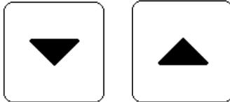
For shades and windows, the **Down** and **Up** buttons are fitted with automatic time functions. The drive can be precisely positioned with brief button presses (less than 1 second, short audio signal). If the button is pressed for longer than 1 second (higher audio signal: locking signal), the drive moves independently to the end position. A brief press in the opposite direction stops the drive.
