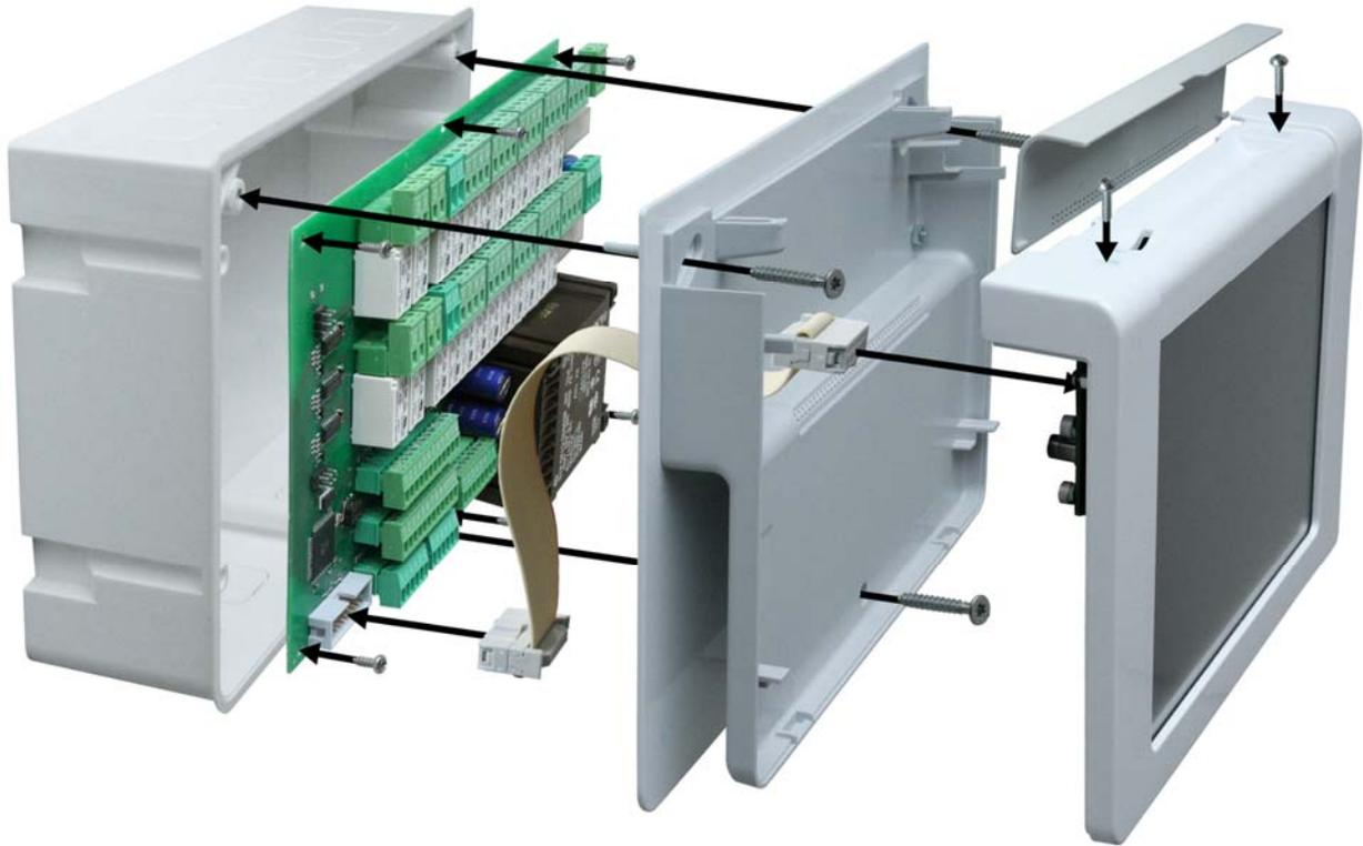
After connecting the cables connect the earth of the wall-mounting plate. Screw the lower section of the housing (with the mounting plate) onto the concealed box. Connect the flat ribbon cable to the display. Put the lid cover on the upper section of the housing (frame with display). Put the upper section of the housing onto the lower section of the housing from above and move it downwards until the bottom edges are aligned. Screw on the upper section.
