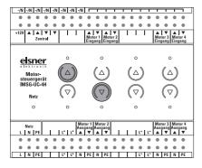
Press the  $\triangle$  button of channel 1 and the  $\nabla$  button of channel 2 for 5 seconds at the same time
