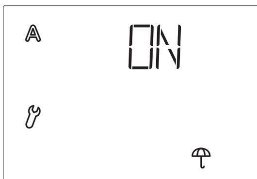
The rain alarm protects shades which are mounted outdoors, especially awning cloth, from damage. When the rain alarm is triggered, the shades are automatically retracted, and manual operation is disabled.
