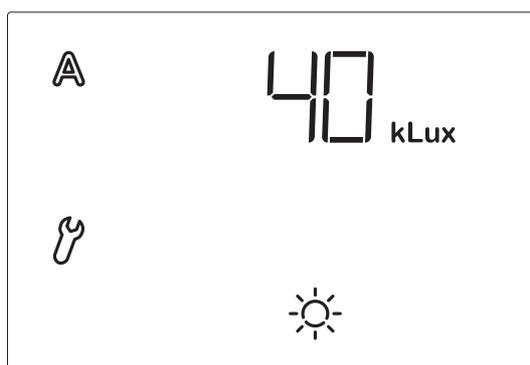
Solar intensity is displayed in Kilolux (kLux). The value 1 kLux is reached already with an overcast sky, at 20 kLux the sun starts being visible, and 100 kLux is reached during a cloudless sky at midday.
