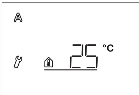
As soon as this value is exceeded, the Automatic function opens the window (unless the outdoor temperature guard value drops below limit, see the next parameter).
