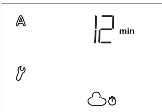
The default setting for retraction is 12 minutes. Brightness must remain below its set value (item A of Automatic settings) for the following 12 minutes in order to retract the extended shades. The dazzle from clouds passing in front of the sun can thus be "blended out".
