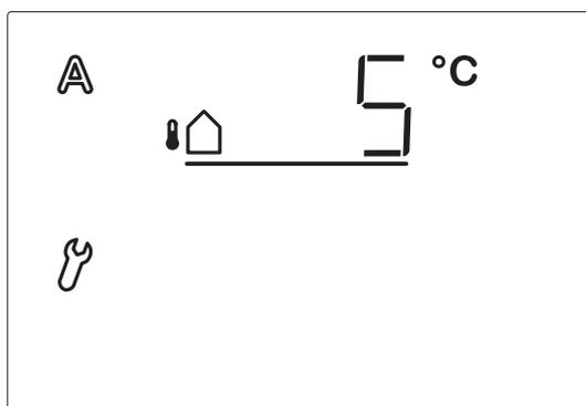
The outdoor temperature guard is important when solar protection equipment is mounted outdoors. Frost can freeze awnings or blinds in their rails. Moving these shades can then damage them.
