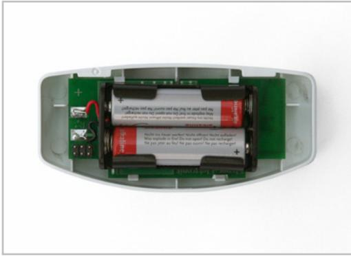
Check that the polarity of the batteries is correct. Two commercially available AA type (Mignon/ LR6) batteries (1.5 V) or rechargeable batteries (1.2 V) are required.
