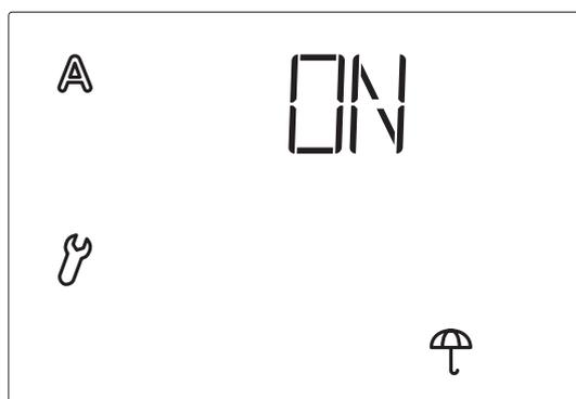
The rain alarm protects the fixtures from damage. When it rains, the window is automatically retracted, and manual operation is disabled.
