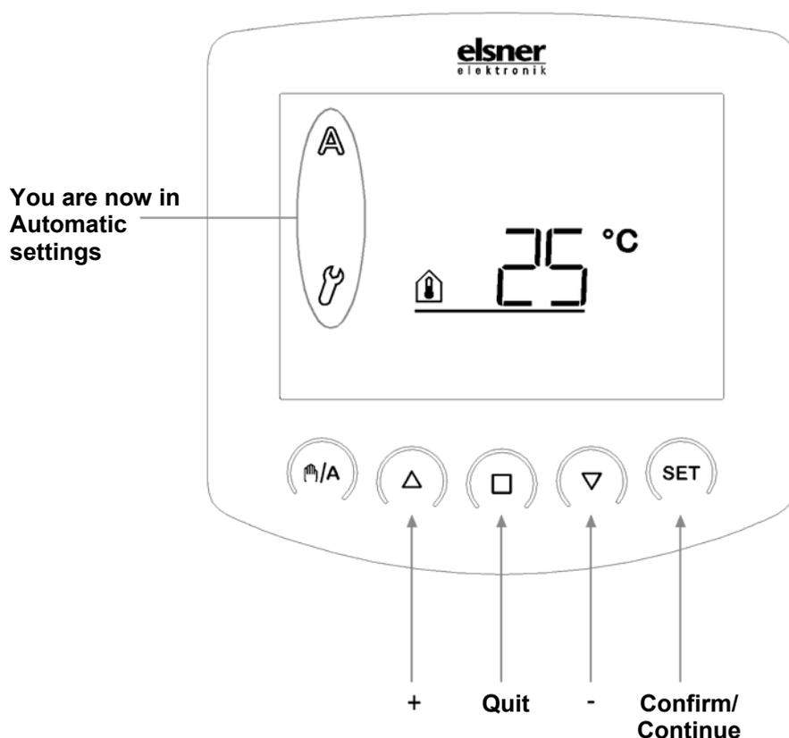
You can exit Automatic settings at any time by pressing the
