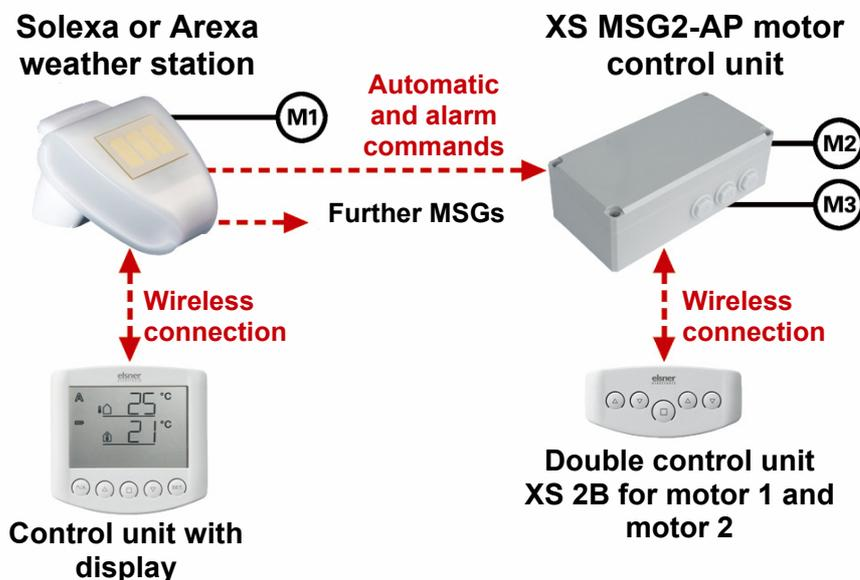
The central control system is suitable for use with drives of the same type, e.g. for awnings only, blinds only or for windows only. The motors receive your automatic commands centrally from the weather station and can be individually and manually actuated using the XS 2B double control unit.
