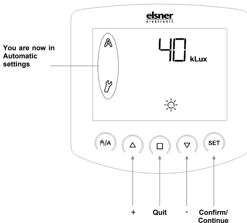
You can exit Automatic settings at any time by pressing the
