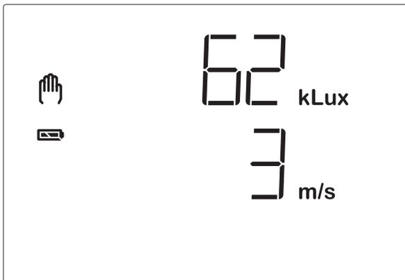
Note: In the first approx. 90 seconds or so following the resumption of voltage to the weather station, the wind value will not be displayed correctly (such as following a power failure, or during commissioning). When the wind alarm is switched on, manual operation is thus disabled in this interval.
