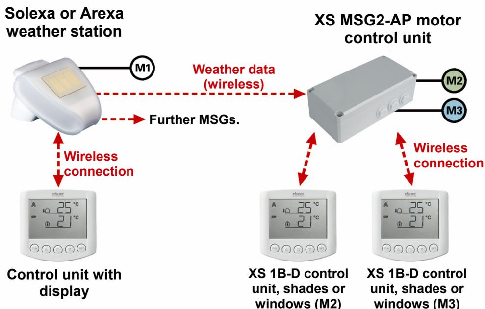
Individual automatic control allows the connection of different drives, such as an awning to weather station, or a blind or a window to a motor control unit. Each drive has its own automatic control, which can be set using the XS 1B-D wireless control unit with display.
