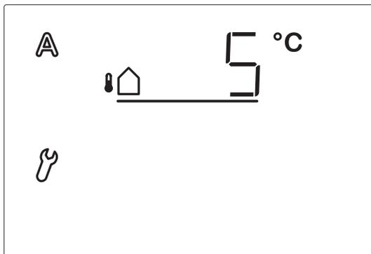
The outdoor temperature guard keeps the window closed when below the selected temperature. This means that in automatic mode, an opened window is closed and is not then re-opened when the indoor temperature value (chapter A) is exceeded.
