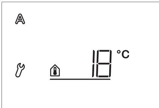
You can use the warmth of the sun with the help of the indoor temperature guard to obtain the desired room temperature (such as in winter). Only once this value is exceeded will the sun trigger the shades.
