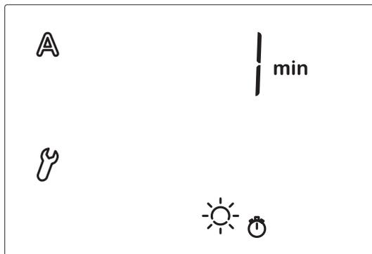
This delay ensures that the shades do not continuously retract and extend in rapidly changing light conditions.
