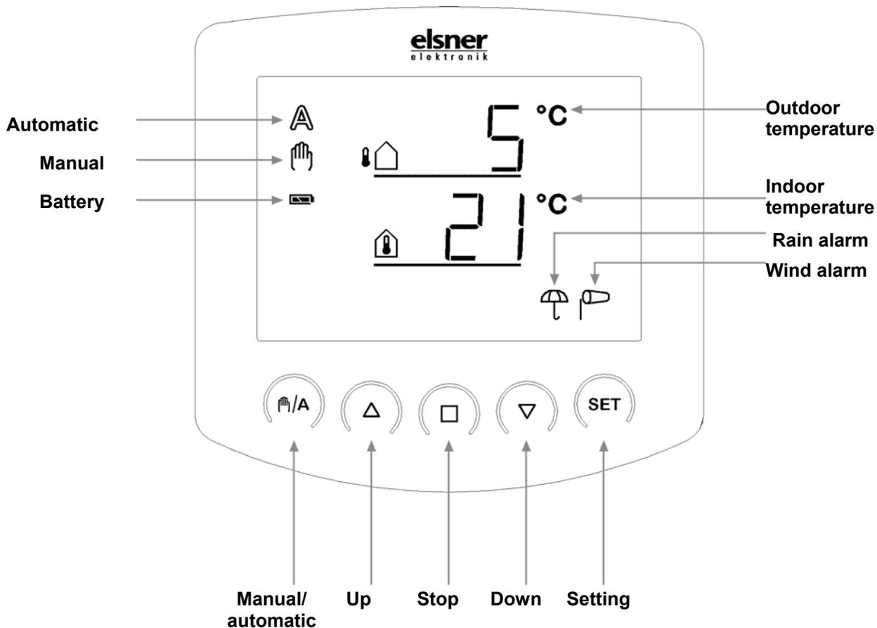
In its initial position, the control system's control unit displays the current outdoor temperature (upper row) and indoor temperature (lower row), as well as the function mode (automatic or manual), battery status and current alarm messages for rain or wind. Weather data is updated once per minute (as well as upon any button press).
