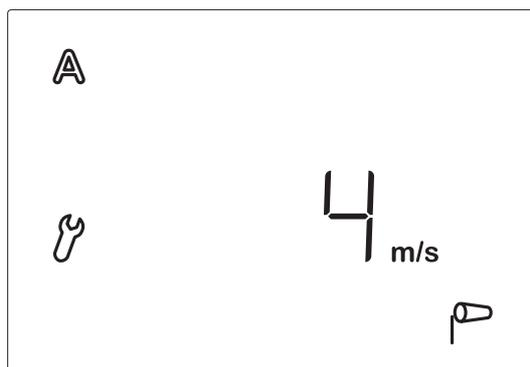
The wind alarm protects the window and fixtures from damage. If the set wind value is exceeded, the window is closed, and manual operation is disabled.
