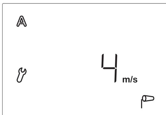
The wind alarm protects shades which are mounted outdoors from damage. If the set wind value is exceeded, the awnings or blinds are retracted and manual operation is disabled.
