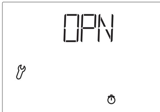
Now open the window as far as the automatic process shall later do (using the  $\Delta$  button).
