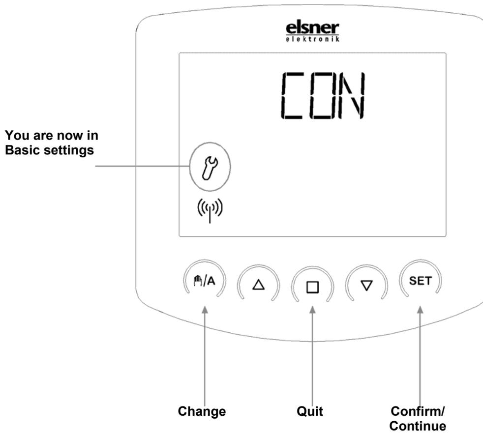
You can exit Basic settings at any time by pressing the  button. The changes which have been made will not then be saved.
