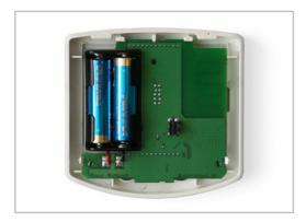
Observe the correct polarity of the batteries. You need two standard batteries (1.5 V) or accumulators (1.2 V) of type AA (Mignon/ LR6).
