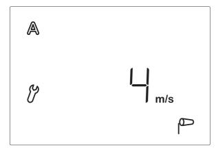
The wind alarm protects the window and furniture and fixtures from damage. If the indicated wind value is exceeded, the window closes and the manual operation is blocked.
