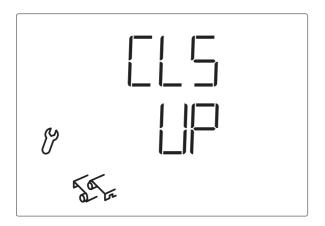
If the up and down connection cables have been mixed up when connecting the drive mechanism, this may be corrected in this step. First open the window a little bit for the rotational direction test. Check both arrow keys and make a setting in the display, whether the window closes again with  $\nabla$  or with  $\Delta$ .
