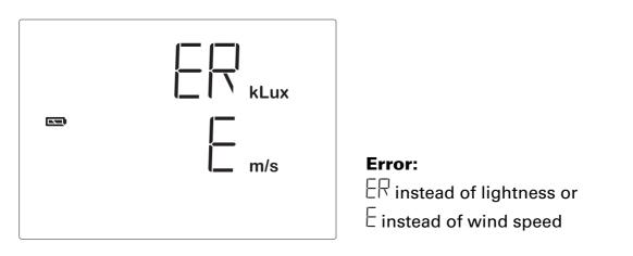
Cause: Lightness sensor or wind sensor of the weather station are defect.
