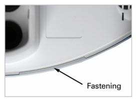
Check whether cover and bottom are correctly engaged! The figure illustrates the closed weather station from below.
