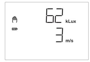
Note: During the first approx. 90 seconds after the return of voltage at the weather station, the wind value is not displayed correctly (e.g. after a power fail or in case of a first start). Therefore, manual operation is blocked in this period of time in case of activated wind alarm.
