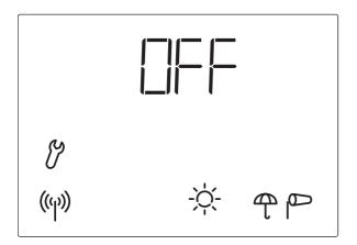
Leave this display at  $\Box \vdash \vdash$  if Arexa is used as conventional single-channel control system. The function "Sending of weather and automatic data" must only be activated if Arexa shall cooperate with motor control devices (e.g. XS MSG2-AP) in the control system XS.
