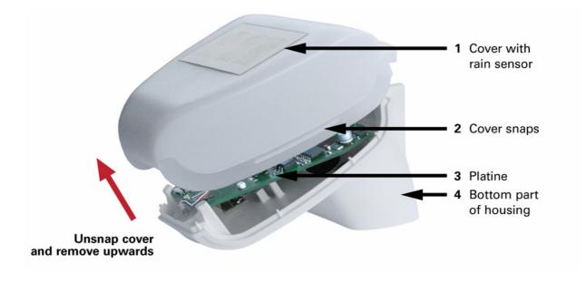
The cover of the weather station with rain sensor is engaged at the lower rim to the right and to the left (see fig.) Remove the cover from the weather station. Be careful not to break away the cable connection between the circuit board in the bottom part and the rain sensor in the cover.
