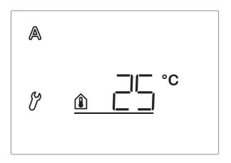
As soon as the value indicated here is exceeded, the automatic opens the window (unless the blocking value for the outdoor temperature has fallen below, see next parameter)
