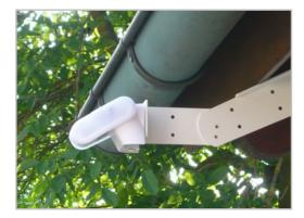
Ex.1: With the hinge arm mounting, the weather station projects from beneath the roof. Sun, wind and precipitation can be measured unhindered by the sensors.
