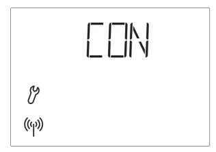
The teaching in may only be accomplished by a qualified person for electronics because the programming key is inside the weather station.
