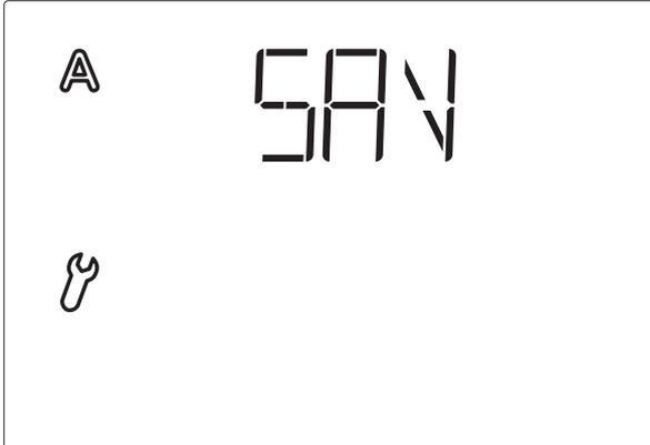
Press the **SET** key in order to save your entered data and to access the meteorological data display. With , you quit the automatic settings without saving.
