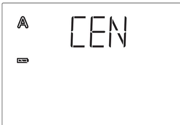
In order to get to the display, press key
