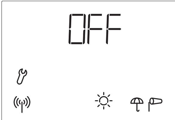
Leave this display at **OFF** if Solexa is used as conventional single-channel control system. The function „Sending of weather and automatic data“ must only be activated if Solexa shall cooperate with motor control devices (e.g. XS MSG2-AP) in the control system XS.
