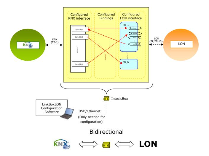
Full and transparent integration of KNX installations (lighting control, window blinds control...) into LonWorks based building management systems (TAC, Kieback&Peter...) now is possible with this powerful and cost effective solution.
