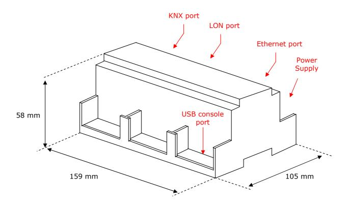
Recommended available space for its installation into a cabinet (wall or DIN rail mounting), with space enough for external connections
