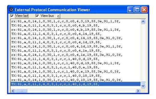
In case there is no response from the Modbus devices to the frames sent by IntesisBox, check that they are operative and configured with the correct communication parameters, check the IntesisBox's Modbus interface connection. See details for the communication cable between IntesisBox and Modbus devices in section *Connections* of this document.
