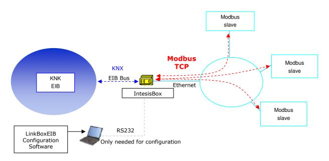
Integration of Modbus and KNX using IntesisBox-KNX Modbus TCP master gateway
