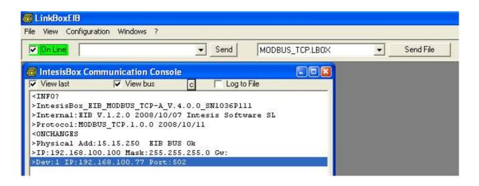
Once connected to IntesisBox, all the options of LinkBoxEIB are fully operative.
