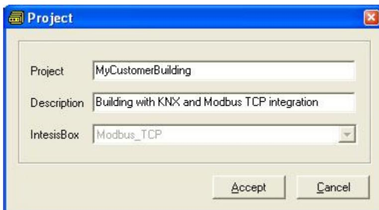
On *Accept*, a new folder will be created inside the projects folder with the name given to the project, this folder will contain the template configuration files if the project is a brand new one, or a copy of the configuration files if it is a copy of a selected one.
