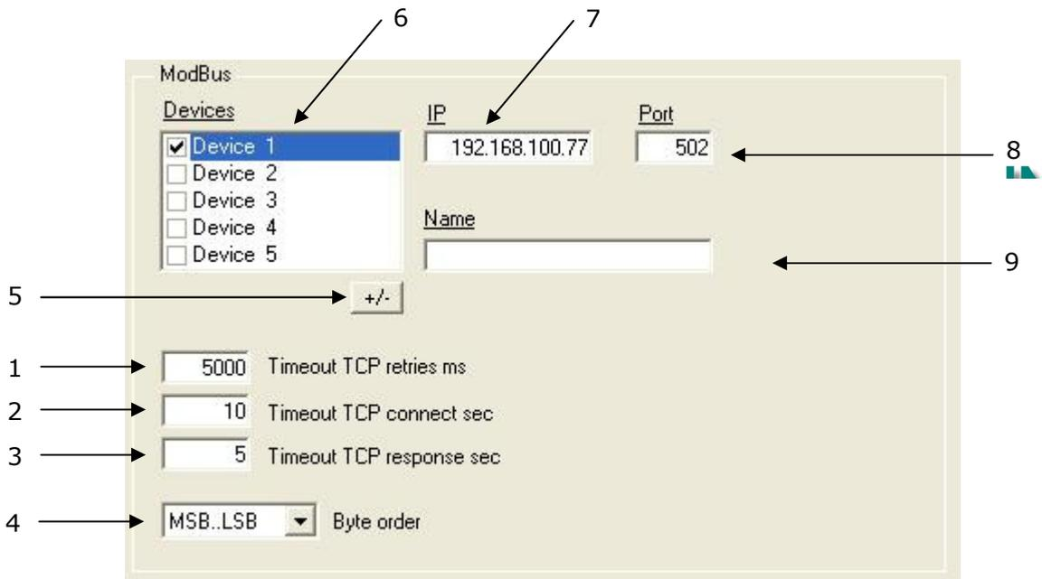
1. Timeout between TCP connection retries (from 100 to 30000 milliseconds).
