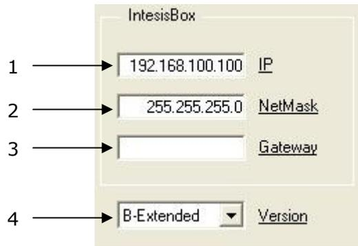
1. Enter the IP address desired for IntesisBox.
