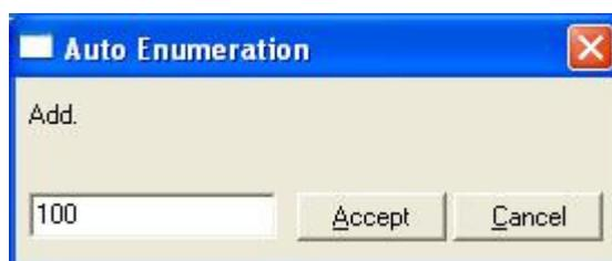
4. Enter the increment between consecutive assignments. For example selecting 100 for the first value and an increment of 1, the values generated will be 100, 101, 102, 103, 104.. and so on. To assign the same value to all the rows (useful to assign the same Device number in the column *Dev* for some consecutive rows) just select the desired value and an increment of 0.
