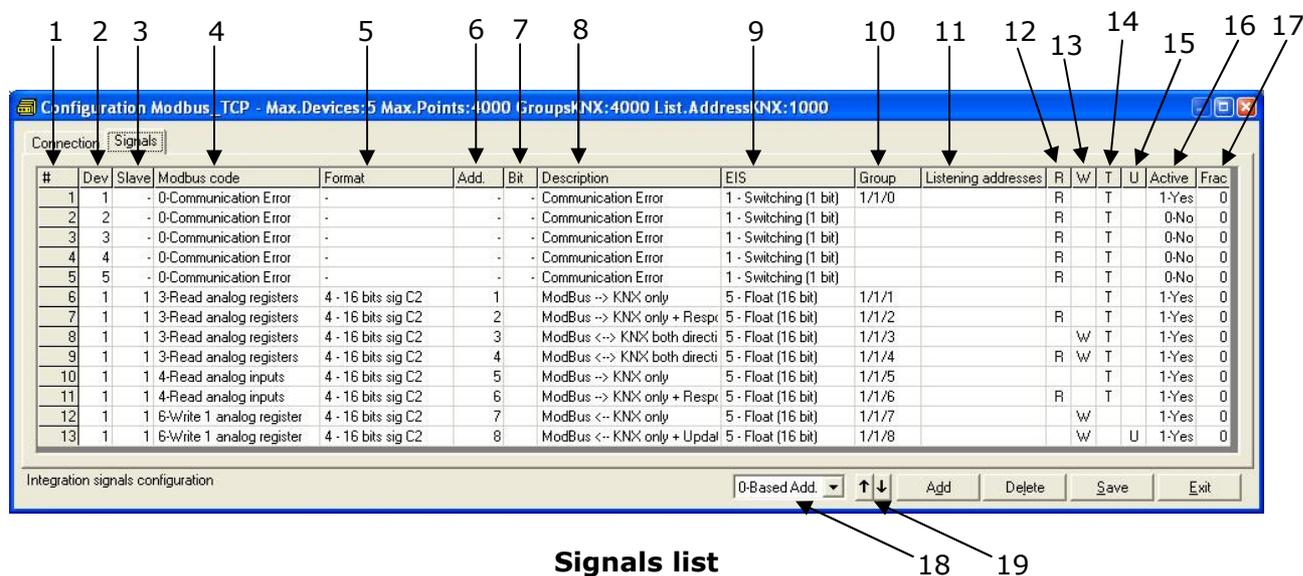
1. #. Signal's number (edit not permitted). Every row in the grid corresponds to a signal (point). Signals (rows in the grid) can be added or deleted selecting the desired row and clicking *Add* or *Delete* buttons. Deletion action can be executed for a single row or even for some consecutive rows, all the rows selected will be deleted. This column is used only to enumerate the rows in the grid (signals).
