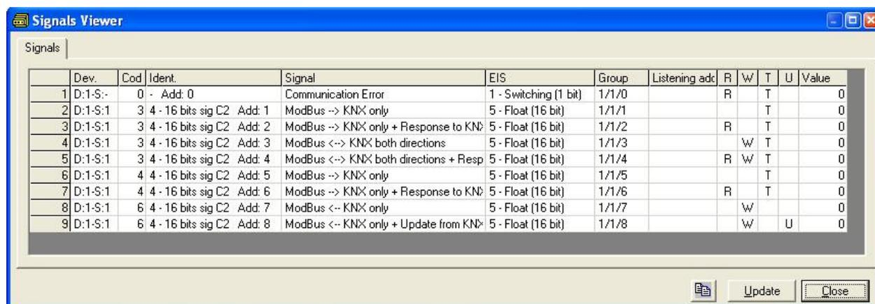
The signals viewer can be used although only one system is connected to the IntesisBox, *KNX* or *Modbus*, and is very useful for supervision and test.
