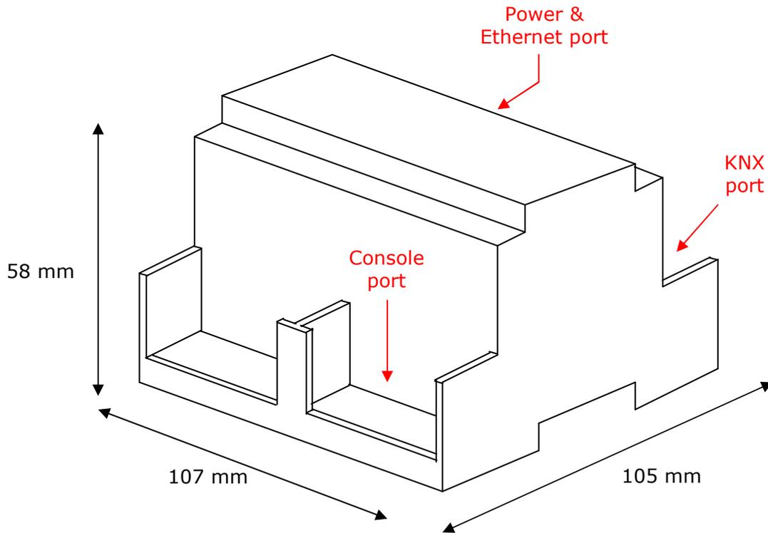
Free space recommended installing the device into a cabinet (wall or DIN rail mounting), with spacing enough for external connections:
