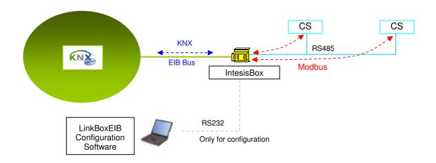
All points of the Airzone system are associated to KNX group addresses, so that the entire Airzone system behaves as one more part of the KNX system with the same configuration and operational characteristics. IntesisBox connects directly to the EIB bus, by its internal opto-isolated bus coupler, and behaves as one more devices into the KNX system.
