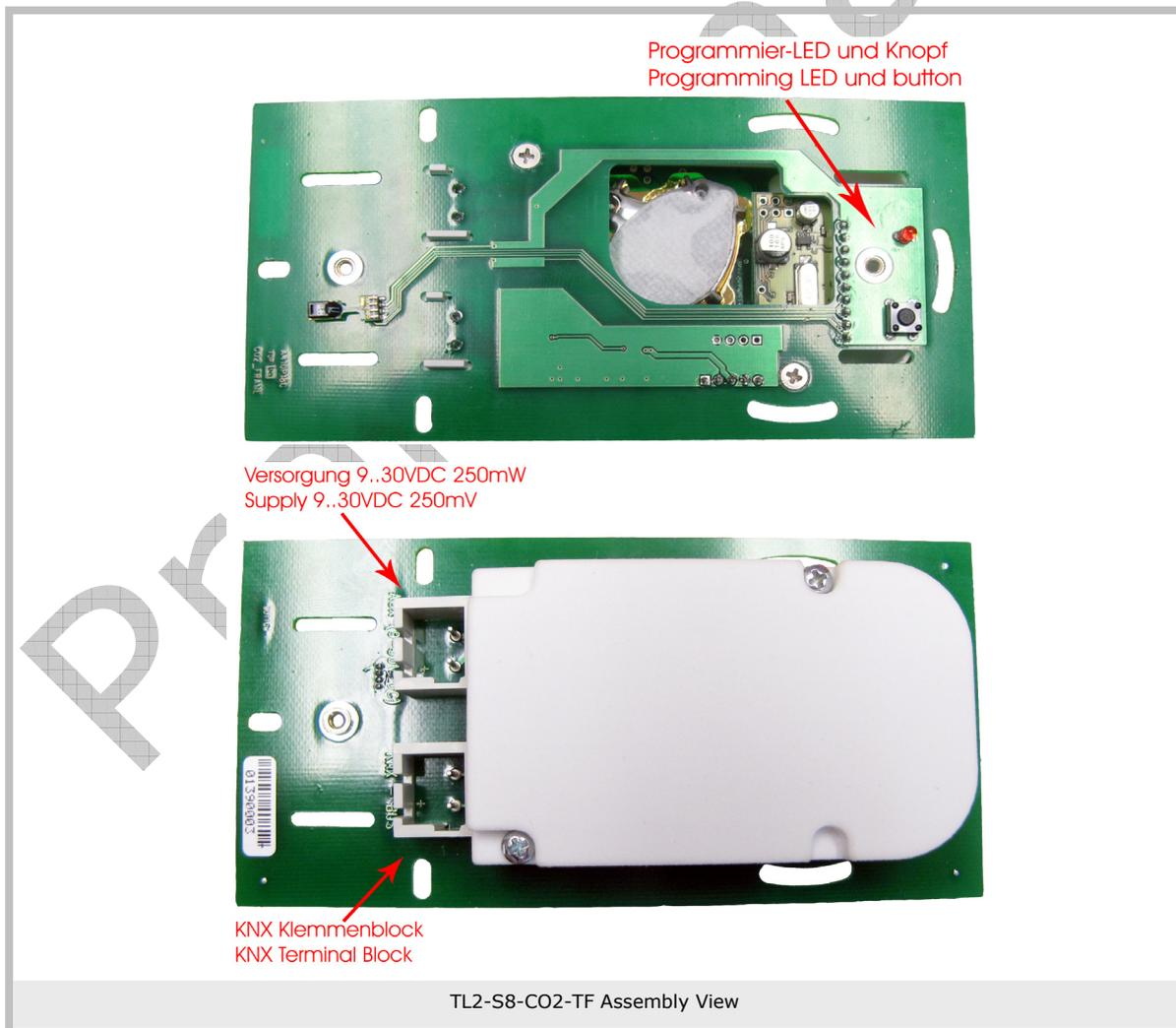
→ Be careful not to damage the electronics with tools and cable heads.
