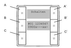
The two rows of the selected function and the associated LED show the value to be sent with the schedule entry. The middle two rows of the text display show the number of the (first) schedule entry, the time and the week days for execution of the schedule entry for this function.
