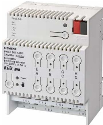
The switching actuator N 567/11 is an N-type device for DIN-rail mounting. With its eight relay contact outputs (channels) it can switch eight groups of electrical consumers independently of each other. The connection to the bus line can be carried out either via a bus terminal block or by a contacting system to a data-rail installed in the DIN-rail.
