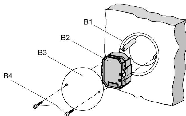
Figure 2: Mounting the binary output UP 562/11
