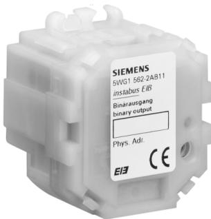
The binary output UP 562/11 is a box mount switching actuator (60 mm Ø, depth 60 mm, a.s.o.). The box mount has to be covered with a universal-cover (ordering separately). Via its 2 outputs it can switch 2 separate groups of electric devices. The load circuits are connected via screwless connection blocks and the EIB bus line is connected via screwless plug-in connection blocks. The binary output UP 562/11 consists of the device (hardware) and its application programs (software).
