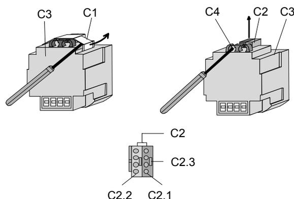
Figure 3: Mounting the binary output UP 562/11
