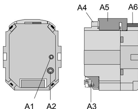
Figure 1: Location of the display and operator elements
