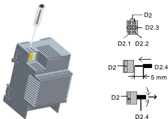
Figure 8. Connecting the twisted pair T+ / T-
