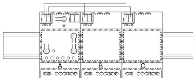
Figure 7. Connecting universal dimmer submodules
