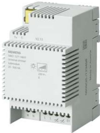
The universal dimmer submodule N 527/41 is an installation device for DIN-rail mounting, with N-system dimensions. It is designed for lighting control, i.e. for switching and dimming resistive, inductive or capacitive loads from 20 to 500 VA at 230V AC, 50-60 Hz. It is connected to a universal dimmer main module or to a preceding submodule via a low voltage terminal block. The power supply for the electronics is provided by an integrated 230V AC power supply unit.
