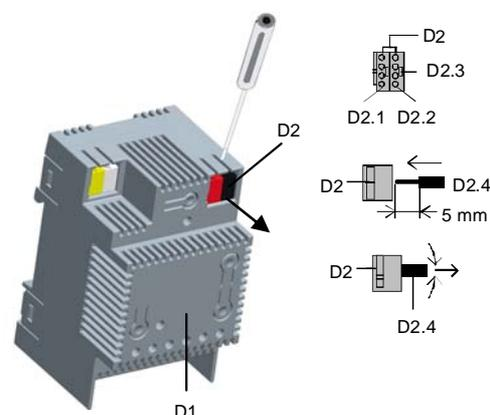
Figure 7. Attaching / removing the bus terminal
