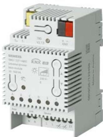
The universal dimmer main module N 527/31 is an installation device for DIN-rail mounting, with N-system dimensions. It is designed for lighting control, i.e. for switching and dimming resistive, inductive or capacitive loads from 20 to 500 VA at 230V AC, 50-60 Hz. The bus is connected via a bus terminal and the power supply for the electronics is provided by an integrated 230V AC power supply unit.
