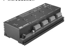
The 4-way universal dimmer is suitable for use with all conventional dimmable types of lighting. There are 4 separate dimmer inputs and outputs, each with a load capacity of 570W. The control circuits automatically detect the connected load, and automatically change over from forward phase control to reverse phase control, and regulate the light output using a suitable control characteristic (Ueff).
