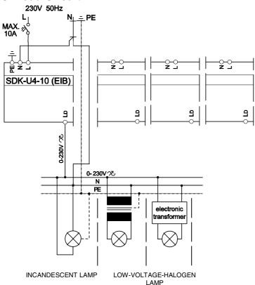
The 4-way universal dimmer is capable of controlling 230V incandescent lamps, low voltage halogen lamps with electronic or magnetic transformers up to a maximum current of 2.5 A (570 W). The dimmed voltage is present at output "LD". The universal dimmer uses transistor circuitry to control the output voltage.
