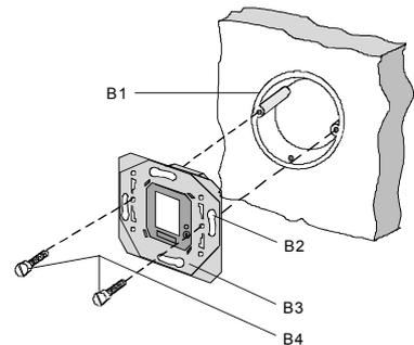
Figure 2: Mounting the dimmer UP 525/21
