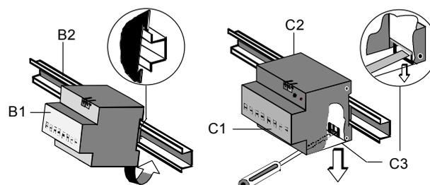
Figure 2: Installing / dismantling the DIN rail mounted device
