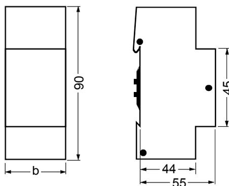
b = 8 module units (1 module unit = 18 mm)
