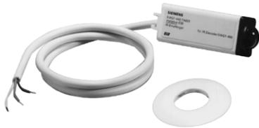
The signals emitted by the IR wall-mounted transmitter are picked up, amplified and converted to electrical signals. These are sent by a three-core wire to the N 450 IR decoder where they are converted into bus-capable telegrams. Within its receiving range, the IR receiver can receive and process the IR signals of all existing transmitters for all the channels occupied in the bus system.
