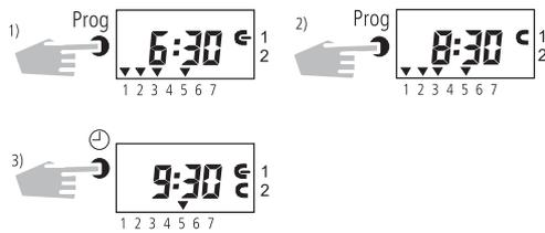
**Illustration 1:** in channel **C1** switch on ( € ) is effected Mo, Tues, Wed, Fri at 6:30 hours
