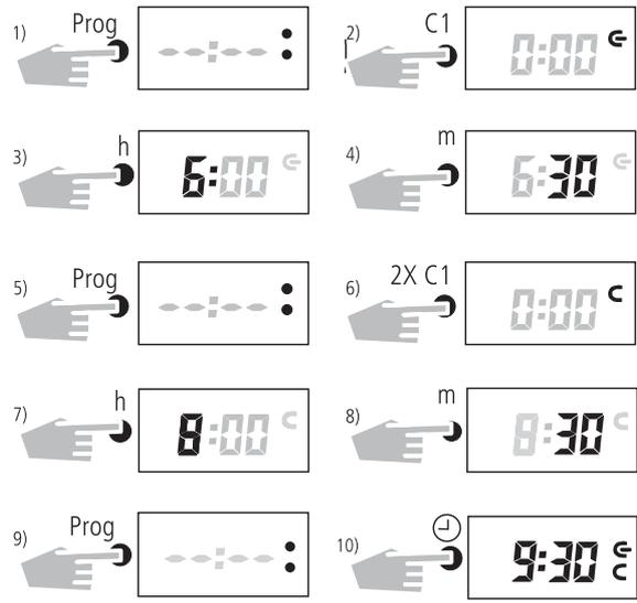
☞ With button **C1** a choice can be made, while programming, whether a switch on (symbol ☞) or a switch off (symbol ☜) should be effected.
