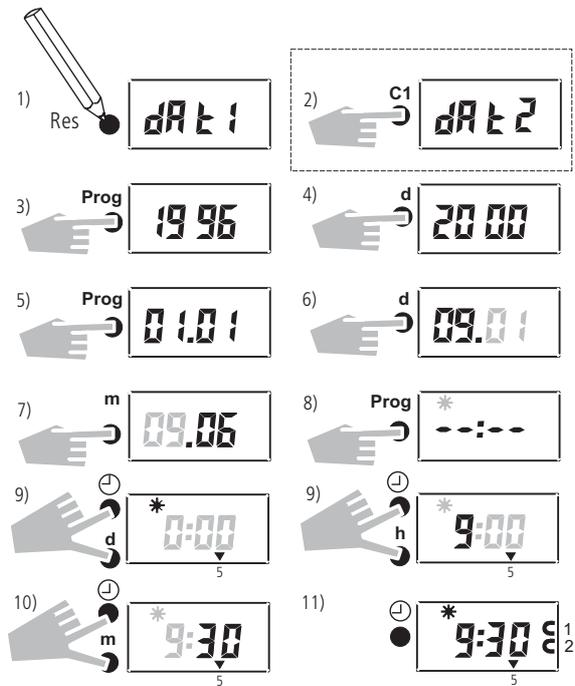
When the button is released after entering the time, both dots between the hour and minute display should flash. If not, repeat the setting.
