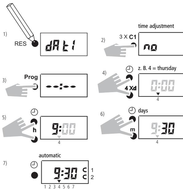
When the button  $\oplus$  is released after entering the time, both dots between the hour and minute display should flash. If not, repeat the setting.
