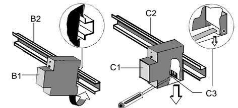
Figure 2: Mounting and dismounting a DIN rail device
