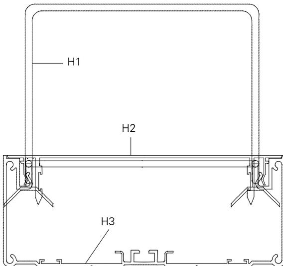
Figure 10: Position of the dismounting hooks (outline section)
