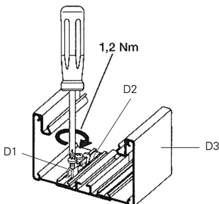
Figure 4: Tightening the earthing clamps
