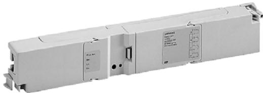
The GE 262 binary input has an oblong design and is therefore suitable for mounting in devices or for separate mounting. Four inputs are available for volt free signalling contacts. The required calling voltage is provided by the binary input GE 262 (no additional power supply required).
