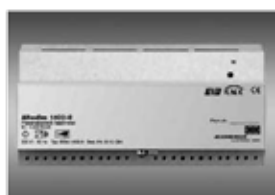
ALTODIM 1400-0 Phase-interval (lagging edge) controlled dimmer for electronic transformers 1400 W/VA
