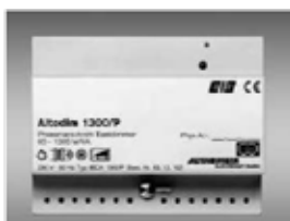
ALTODIM 1300/P Phase-controlled (leading edge) dimmer for incandescent lamps, high-voltage halogen lamps, low-voltage halogen lamps with wire- wound transformers, neon lamps, 1300W/VA
