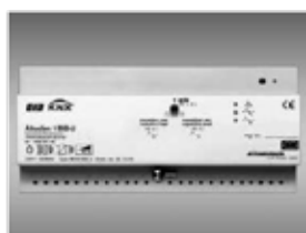
ALTODIM 1500 U Universal dimmer for electronic transformers, incandescent lamps and low- voltage halogen lamps with wire-wound transformers, 1500W/VA
