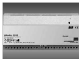
ALTODIM 2000 Phase-controlled (leading edge) dimmer for incandescent lamps, high-voltage halogen lamps, low-voltage halogen lamps with wire- wound transformers, neon lamps, 2000W/VA
