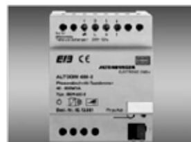
ALTODIM 600-0 Phase-interval (lagging edge) controlled dimmer for electronic transformers 600 W/VA
