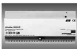
ALTODIM 2000/P Phase-controlled (leading edge) dimmer for incandescent lamps, high-voltage halogen lamps, low-voltage halogen lamps with wire-wound transformers, neon lamps, 2000W/VA
