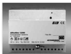
ALTODIM 1300 Phase-controlled (leading edge) dimmer for incandescent lamps, high-voltage halogen lamps, low-voltage halogen lamps with wire- wound transformers, neon lamps, 1300W/VA
