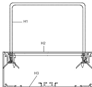
Figure 10: Position of the dismantling hooks (outline section)
