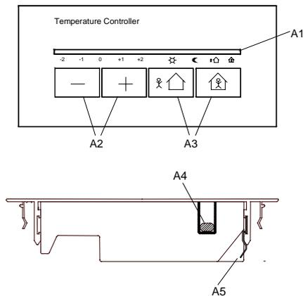
Figure 1: Location of the Display and Operator Elements
