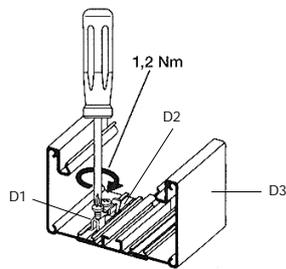
Figure 4: Tightening the earthing clamps
