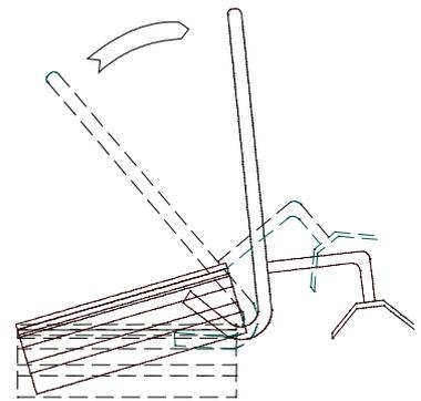
Figure 11: Levering out the channel unit's top part respectively the modules
