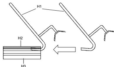
Figure 9: Putting the dismantling kit to the dismantling position for channel top parts (side view)
