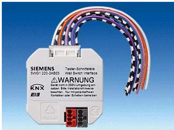
The push button interfaces UP 220/03 and UP 220/13 are binary input devices for use with box mounts (∅ 60 mm, depth: 40 mm). Four/two inputs are available for potential-free switch/push button contacts. The required scanning voltage is provided by the push button interface (requires no additional power supply).
