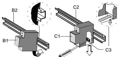
Figure 2: Mounting and dismounting a DIN-rail device
